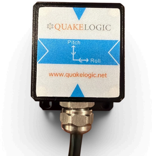
QL-MODALINK node: IP68 aluminum housing with sealed cable gland.
