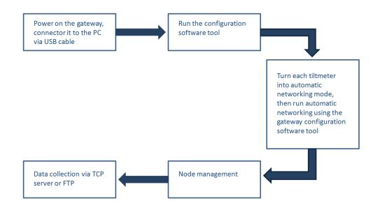
The above figure shows the general operating process for collecting data from the tiltmeters via the gateway.
