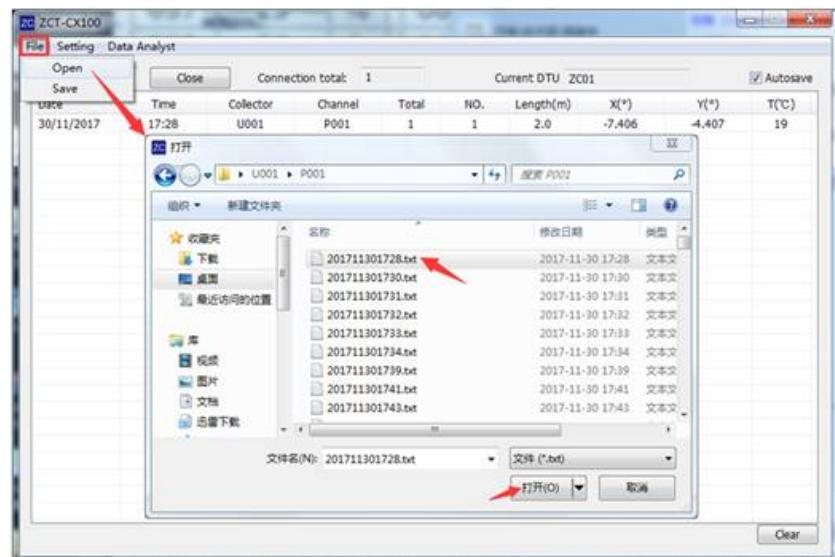
C) If the upper computer is down for a period of time, after the repair, the microSD card on the datalogger can be taken out and loaded into the card reader connected to the computer. The upper computer can open the file stored in the card for backup so no monitoring data is lost.
