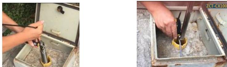
6.3 Connect the remaining probes one by one.
