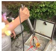
6.2 Hang the probe on the wellhead with a screwdriver or other tools, install the connecting rod, and tighten the locking bolt.
